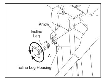
After you have adjusted the incline legs, lower the treadmill (see HOW TO LOWER THE TREADMILL FOR USE on page 15).
